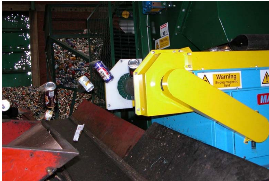
Exhibit 6. Eddy Current Separator for Non-Ferrous Metals
