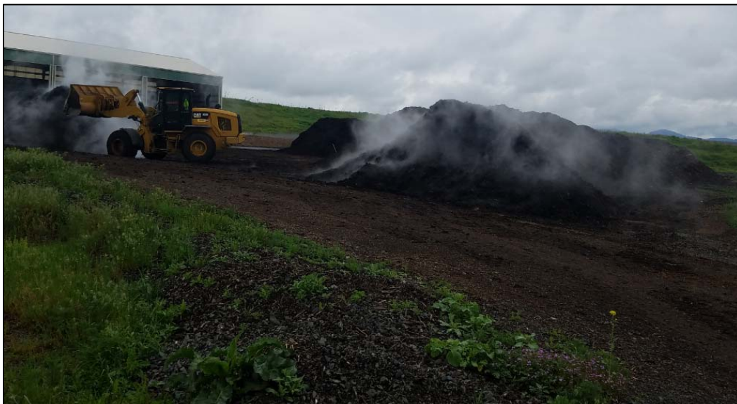
Exhibit 7. Curing Compost Piles at the SWPF
