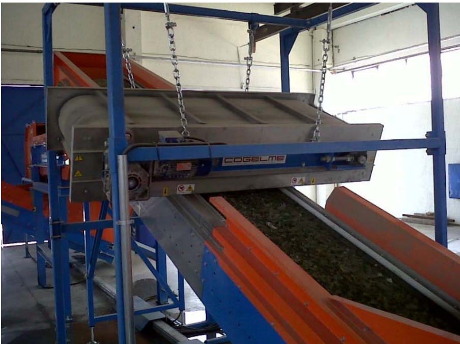
Exhibit 5. Electromagnet Unit for Ferrous Metal Separation
