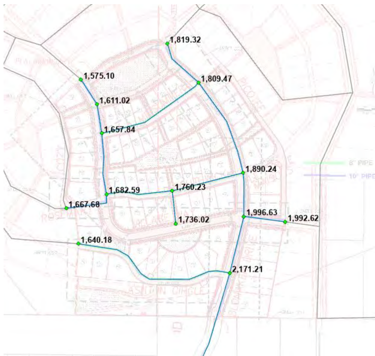
Figure 4. Steady-state available fire flow, part of Main Pressure Zone (gpm)
