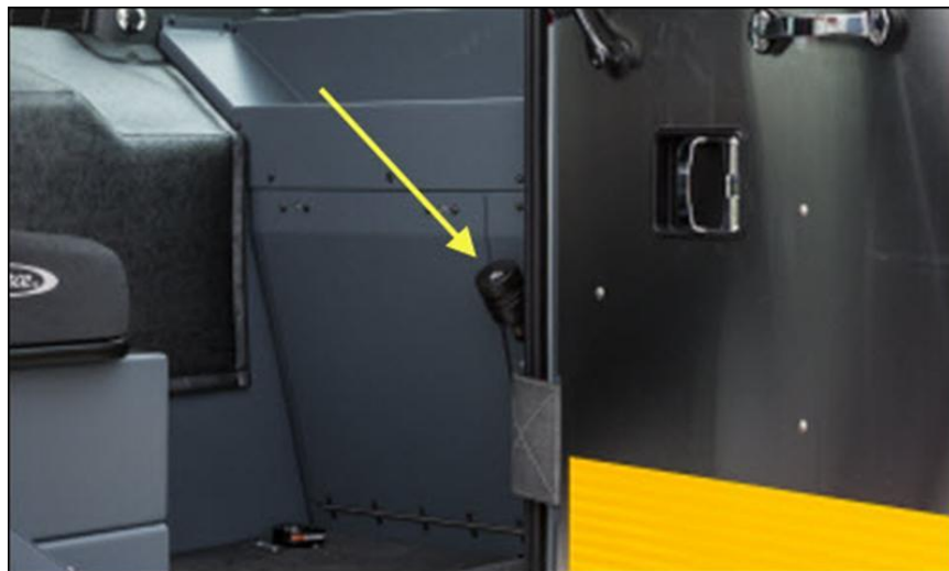
[Washer Reservoir Location]
