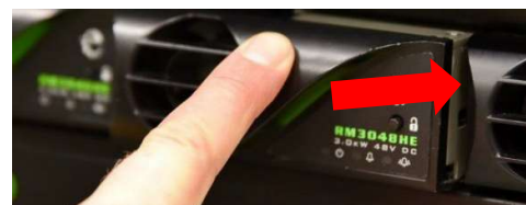
Figure 14: Inserting a Rectifier
